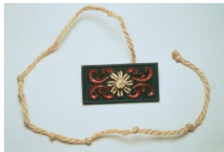
Figure 3: The notched rope ensured that the latitude measurements provided by users of this kamal were consistent.
