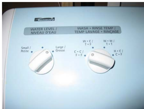
Figure 8: The cold-wash and cold-rinse setting (C-C) means less hot water is used during the wash cycle. The hot-wash, cold-rinse setting (H-C) requires more hot water. If you make sure you wash only large loads (high water setting) the energy savings will be even greater.
