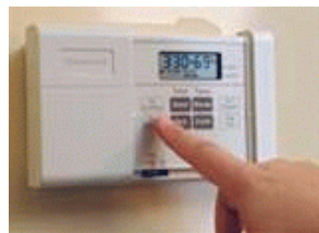
Figure 4: This device allows for real-time monitoring of electricity usage.
