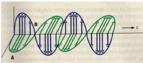
At point A the electric and magnetic fields associated with the wave are at maximum strength and at point B the fields are at minimum strength.
