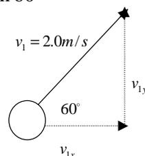
At the peak of its ascent the velocity of the ball in the y-direction will be 0 m/s. The time taken to reach that maximum height can be found from the equation,
