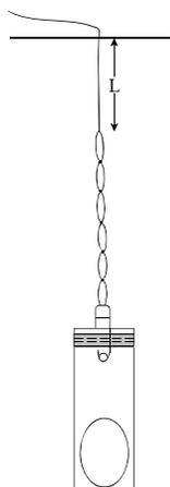
The different maximum distances that the egg falls through are achieved by changing the length of the unstretchable part of the cord, that is, the length between the topmost rubber band and the point where the cord is tied to the support arm. As this distance gets bigger, the egg will fall through a larger distance.
